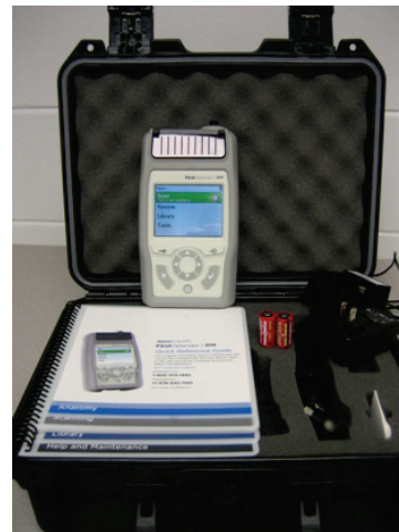
FirstDefender RM in Pelican ® carrying case, with chargers, batteries, and manual (memory card within unit)
