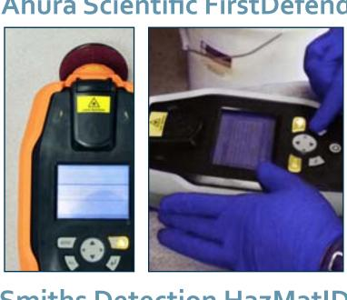
This portable, handheld Raman spectrometer is used to rapidly identify unknown solid and liquid chemical substances, including forensically relevant materials such as controlled substances and ignitable liquids. Raman technology measures the inelastic scattering of monochromatic light, usually from a laser in the visible, near-infrared, or near-ultraviolet range.
