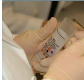
These single-use test ampoules use colorimetric technology to screen substances for the presence of classes of narcotics. Each test kit contains a proprietary reagent-granulate (liquid and crystals) and a band of color to indicate a positive result. The tests are optimized for field use and allow law enforcement officers to presumptively test for narcotics including cocaine and crack cocaine, heroin and methamphetamine.
