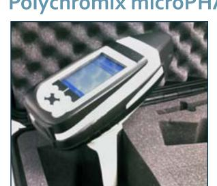
The microPHAZIR<sup>TM</sup> field-portable near-infrared (NIR) spectrometer is used to conduct fast, non-destructive, qualitative or quantitative analysis on solids, powders and other materials used in a variety of industries. The instrument can identify forensically relevant materials such as controlled substances and explosives.
