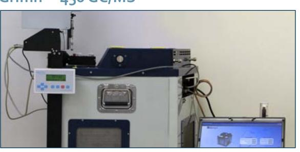
The Griffin<sup>TM</sup> 450 gas chromatography mass spectrometry (GC/MS) chemical analyzer is used to analyze and identify forensically relevant chemical compounds in the field including narcotics, ignitable liquids and explosives. This device, typically found in the laboratory due to its size and power source, has been optimized and ruggedized for field use.
