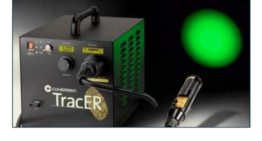
The TracER<sup>TM</sup> is a portable, solid-state argon laser used to detect the presence of fingerprints and trace evidence. The laser uses inherent luminescence or chemical fluorescence to reveal evidence undetectable with the naked eye. The device is lightweight, compact, air-cooled and powered by alternating current or an optional on-board battery for optimal field use.
